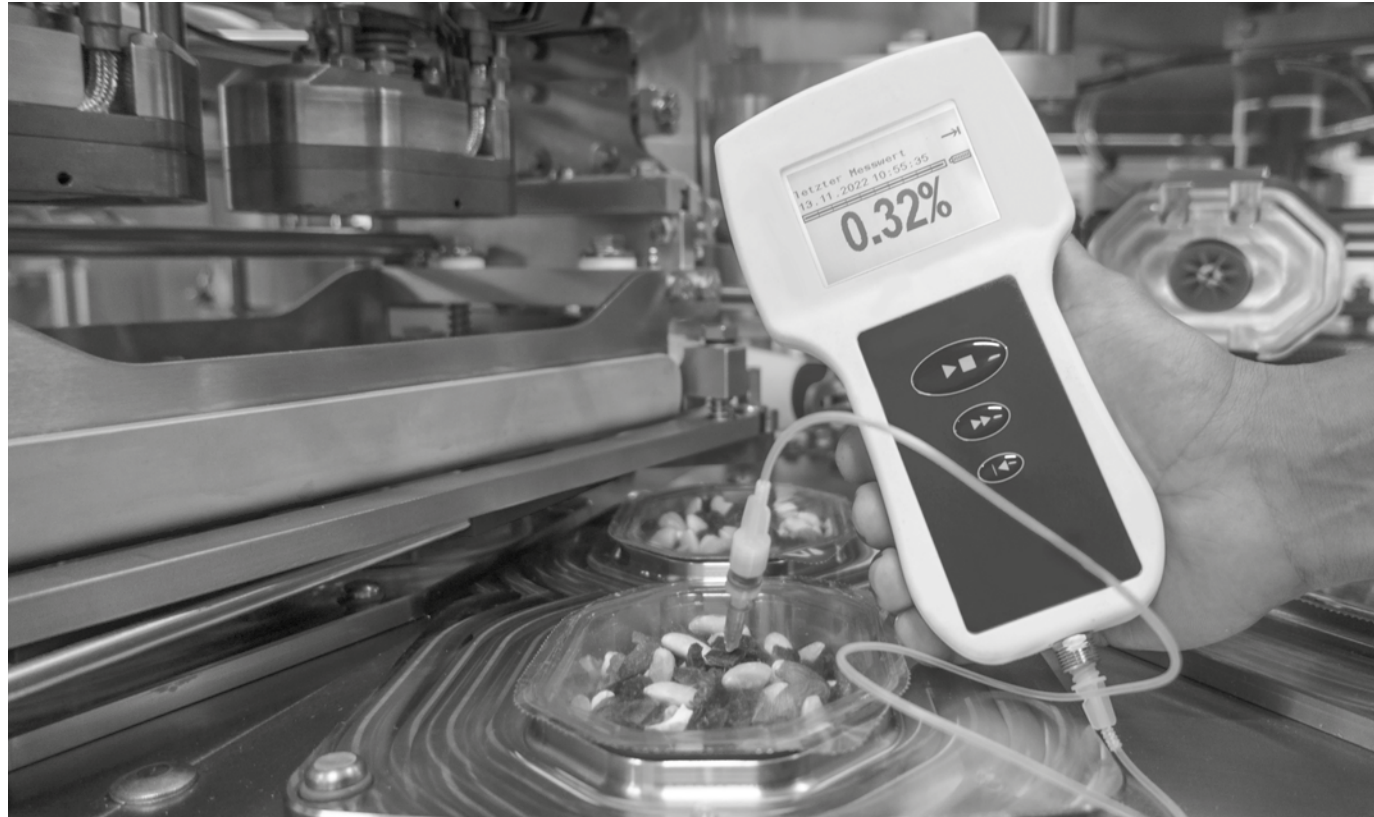
The new Grunwald gas injection system allows for a remaining oxygen content of < 0.5 % at 40 cycles/min.
